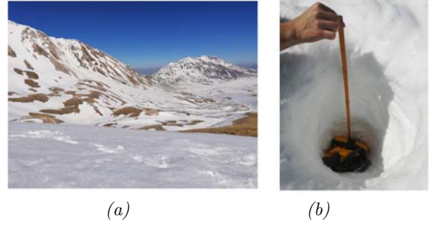
Figure 4. a) Campo Imperatore field on the top of Gran Sasso mountain; b) The 1 m deep hole in the snow used for burying the transmitter inside the watertight bag.
