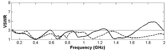
Fig. 9. VSWR of a bifolded monopole with resistors constrained close to the ground plane (Fig. 7). Simulated data (dashed line) are compared with measurements (solid line) on the 1:50 scaled prototype in Fig. 8.
