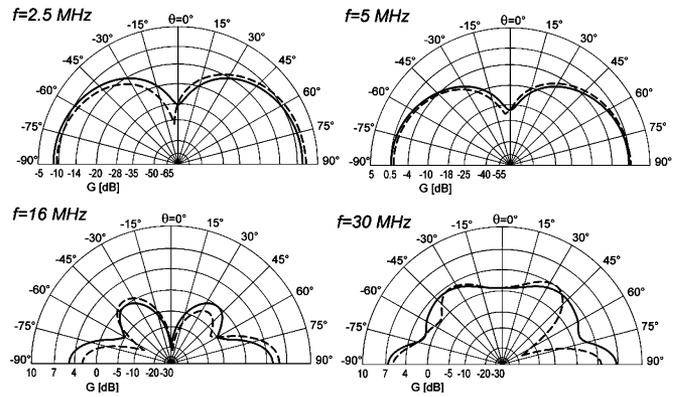
Fig. 6. Radiation patterns at some frequencies. Solid line:  $\phi = 0^\circ$  cut; dashed line  $\phi = 90^\circ$  cut.
