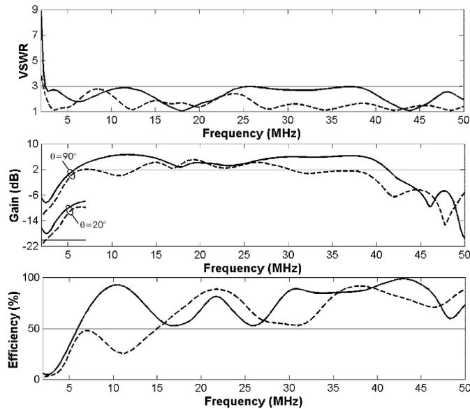
Fig. 4.  $\phi$ -averaged gain at the horizon and at  $\theta = 20^\circ$ , and system efficiency after loading optimization in the range 2–50 MHz. Solid lines tag the bifolded monopole loaded with four circuits, while dashed curves are for the reference folded monopole having the same size of the proposed antenna, and loaded with seven circuits.
