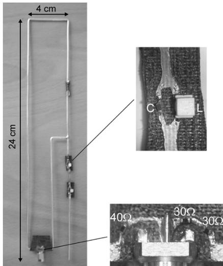
Fig. 8. Scaled model (1:50) of the bifolded antenna in Fig. 7. The conductor is a 2-mm diameter copper wire. Loading electric devices are sustained by a dielectric substrate. On the right, some details about the loading circuit realization: the 60- $\Omega$  resistor has been obtained as series connection of two 30  $\Omega$  ones.
