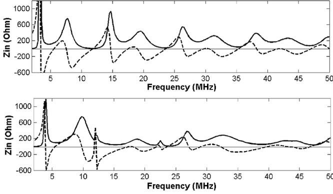
Fig. 2. Input impedance in the range 2–50 MHz of the unloaded folded monopole (up) and of the new bifolded monopole (down) of size in Fig. 1. Solid and dashed lines respectively refer to real and imaginary part of the input impedance.
