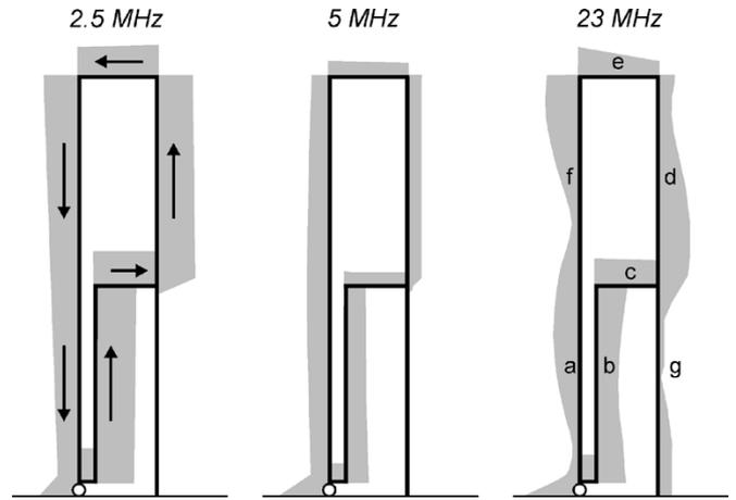
Fig. 5. Current patterns (amplitude) at some frequencies. Arrows indicate the current direction.
