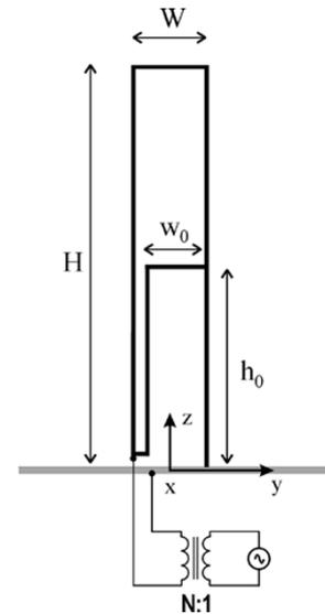
Fig. 1. Geometry of the *bifolded monopole* over an infinite ground plane. The impedance transformer ratio  $N$  will be optimized together with antenna loading. Antenna size:  $H = 12$  m,  $W = 2$  m,  $h_0 = H/2$ ,  $w_0 = 1.6$  m.
