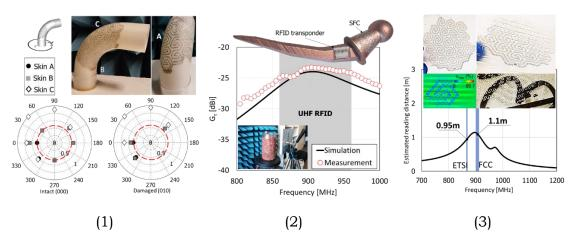
**FIG. 3** – 1) Interruption of SFC due to cracks has an impact over the reading distance. In any case, a 0.5 m reading distance is achieved. 2) Comparison between the simulated and measured realized gain of the prosthesis in the limb mock-up. 3) Prototype of the elastic space filling wireless sensor under two stretch conditions. Numerical mechanical analysis under 35% x-direction stretching and simulated reading range with 3.28 W EIRP.
