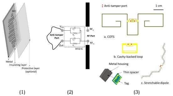
**FIG. 2** – 1) Arrangement of SFC over a metal surface by means of insulated layer. 2) Equivalent circuit to account for the RF coupling between the antenna and the anti-tamper port of the IC. 3) Modularity of the proposed approach. Depending on the environment, it can be a) a COTS module, b) a cavity-backed loop optimized for metal surface proximity or a c) stretchable dipole, for elastomeric surfaces.
