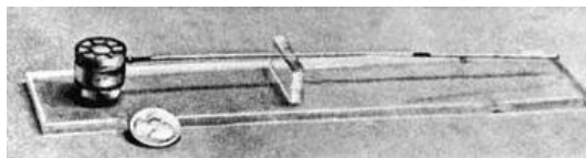
Figure 1: Theremin’s bug (1945), the first passive radio sensor converting voice pressure into a modulation of the radar cross-section of a wire antenna through a capacitor microphone.
