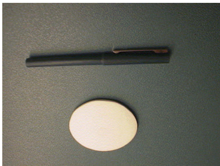
Microwave lens manufactured using glass epoxy
