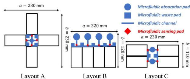
Figure 1. The three considered layouts of the NFC system: layout A, layout B, and layout C. The external size  $\{a, b\}$  for each configuration is reported, as well as the starting geometry for the corresponding microfluidic circuit.
