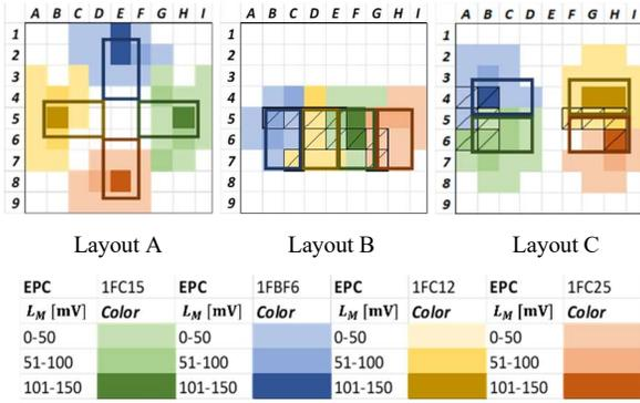
Figure 3. Coverage maps of the three system layouts and measured load modulation, reporting the boards' positioning. Bordered squares denote that two responders communicated in the same area. In no area more than two boards have ever responded.
