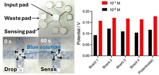
Figure 4. System integration and test for sodium sensing. A zoomed-in picture of the microfluidic and test with *Molybdenum blue* 1 mM are shown on the left.
